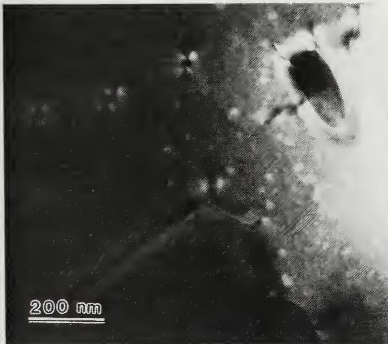
Figure 10B Dark-field TEM Micrograph of 6061 Aluminum Aged for 1200 Seconds at 373K.
